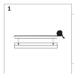
Measure distance between holes for the mounting bracket installation
