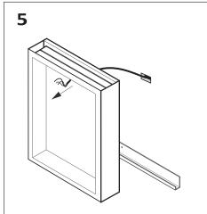
Pull through the electrical wires
