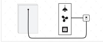
Install optional outside switch to control the defogger Refer to how to use guide for more information
