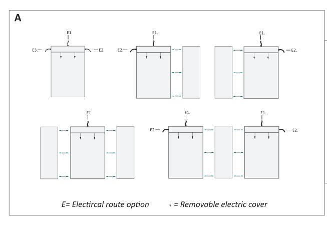
Connect cabinets with connectors provided at top, middle and bottom. Here are some different ways
