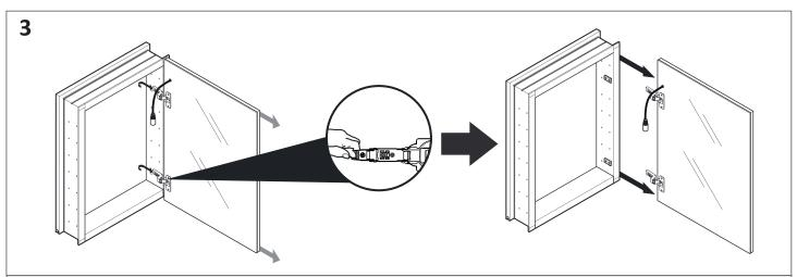
While supporting the door release (the leaver under the hinge arm), slide the door off the frame.
