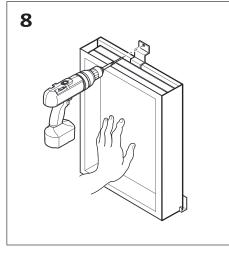
Attach the top mounting bracket to the wall using a screw gun
