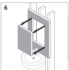
Cut the marked perimeter with suitable tool
