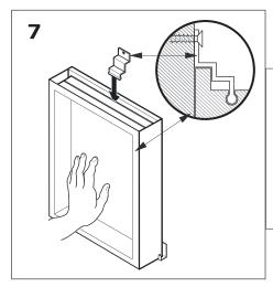
Insert top mounting bracket into the top of the cabinet
