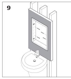
Affix using screws into the studs
