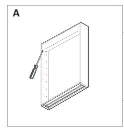
Remove the electric box panel inside the cabinet
