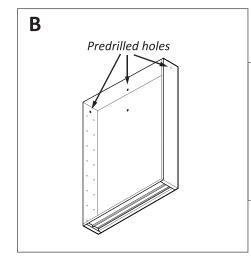
Use optional predrilled holes for electrical connection
