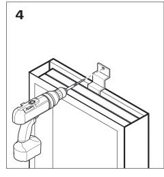
Secure the top bracket to the wall using screw gun
