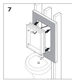
Connect electrical wires before inserting the cabinet into the opening
