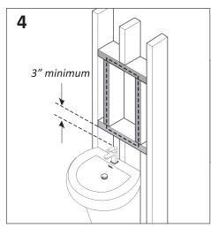
Frame the opening for the cabinet based on the measurement
