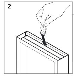
Slide top bracket into the channel at the top of the cabinet
