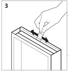
Make sure top bracket is locked in the groove
