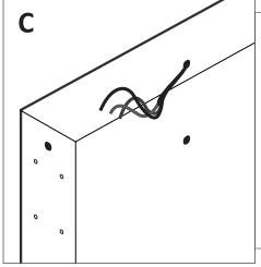
With panel removed change the location of electrical cord according to you electrical needs
