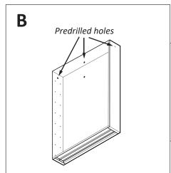
Use optional predrilled holes for electrical connection
