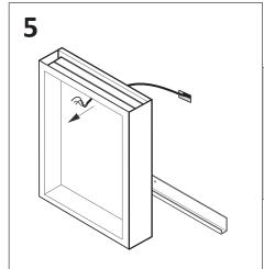
Pull through the electrical wires
