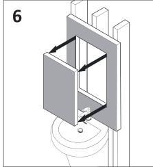
Cut the marked perimeter with suitable tool
