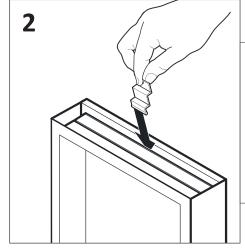
Slide top bracket into the channel at the top of the cabinet
