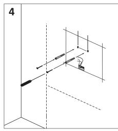
Insert anchors into predrilled holes
