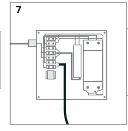
Make the electrical and ground wire connection
