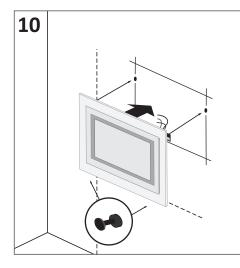
In case of the wall not having an even surface, use the included adjustors on back of mirror
