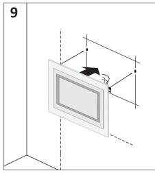
Hang the mirror with care onto the screws making sure it's secure
