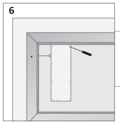
Unscrew the back plate of the electrical box
