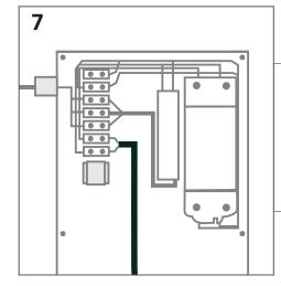
Make the electrical and ground wire connection
