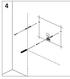
Insert anchors into predrilled holes
