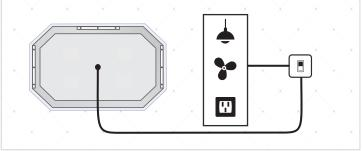
Install optional outside switch to control the defogger Refer to how to use guide for more information
