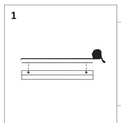
Measure distance between holes for the mounting brackets installation
