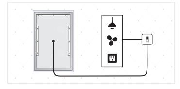
Install optional outside switch to control the defogger Refer to how to use guide for more information
